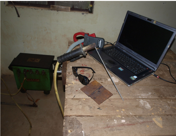
Figure 6: Single phase ARC welding machine setup
